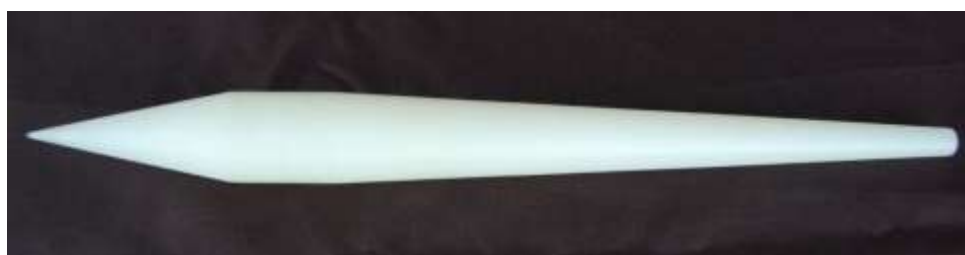
Figure 2: Tapered Nylon dielectric rod antenna ( \theta_0 = 2.5^\circ ).
