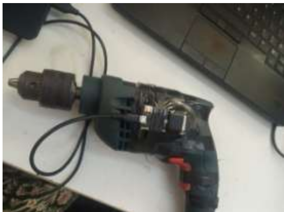
Fig 3. Sensor mounting on drilling machine.
