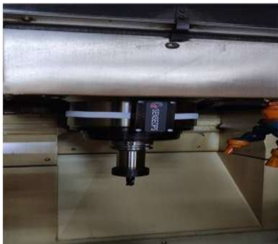
Fig 4. Sensor mounting on CNC drilling machine.
