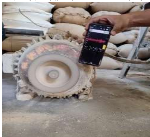
Figure 3: More distortion at low greasing level
