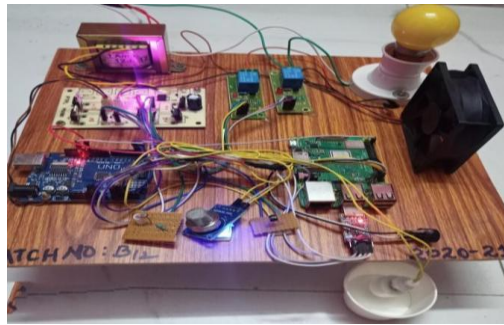
Fig.10 Connecting IoT based industry automation using raspberry pi system
