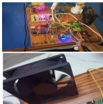
Fig.9 Output of temperature sensor when the room crosses its temperature then fan will automatically gets on
