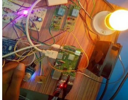
Fig.6 Output of the light sensor when the room gets dark then automatically light gets on
