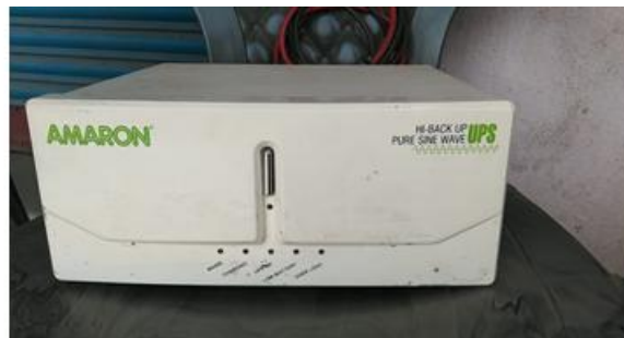
Figure 3: Inverter and charger.
