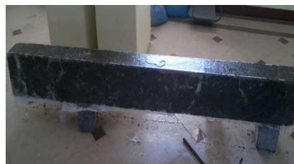
Figure 7: Beam S-1 after U Wrapping and resin application
