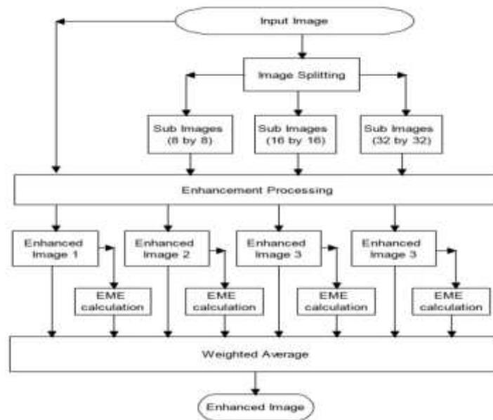
Figure 6:Block diagrams of the proposed algorithm
