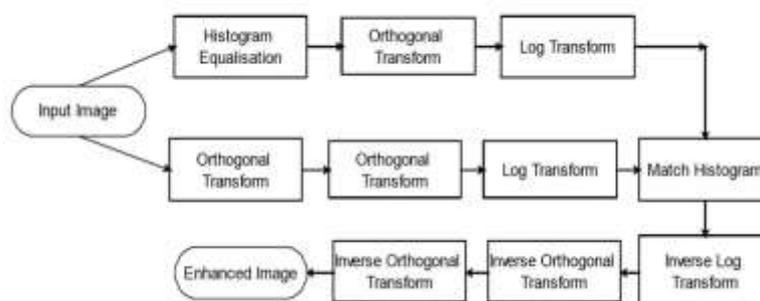
Figure 8:Block diagram of the Enhancement Processing
