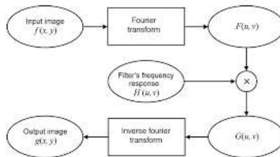
**Figure 5:** Enhancement steps in frequency domain
