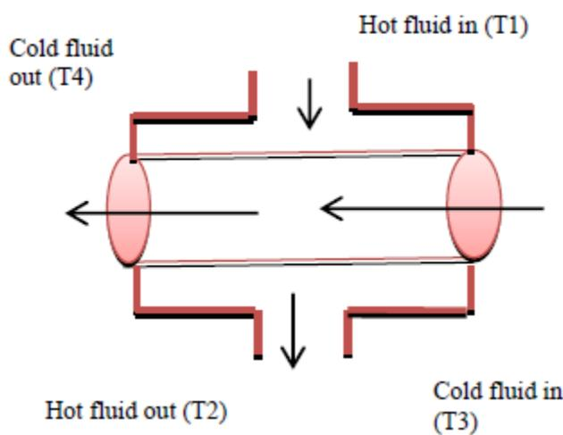
Figure 4: Cross flow heat exchanger
