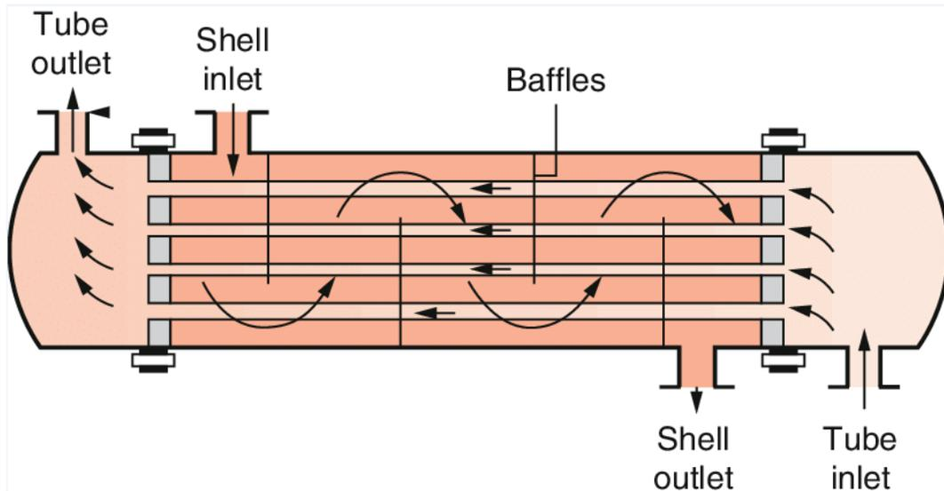
**Figure: 1:** Schematic diagram of a shell and tube heat exchanger with one shell pass and one tube pass
