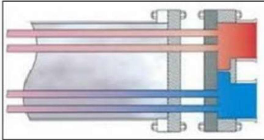
Figure 6: Double Tubesheet
