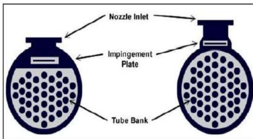
Figure 7: Nozzle Impingement Plate Tube-Side Channel and Nozzles
