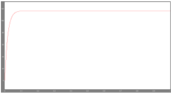
Fig.7: Switched capacitor output voltage
