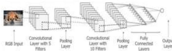
**Figure 2:CNN Architecture**
