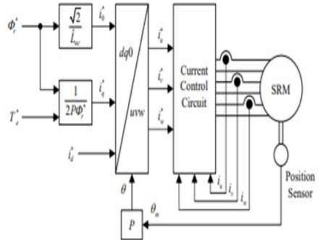
Fig. Vector Control System for SRM Drive
