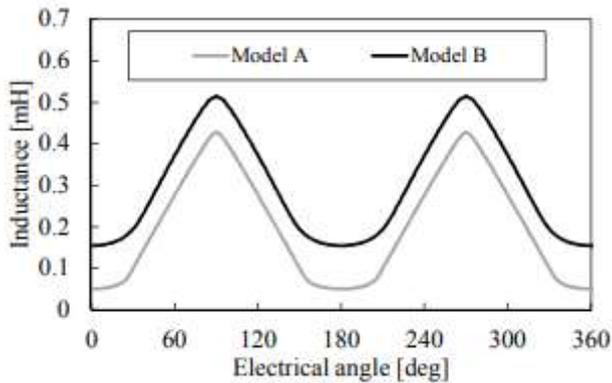
Fig. Self-inductance waveforms of the proposed SRMs.
