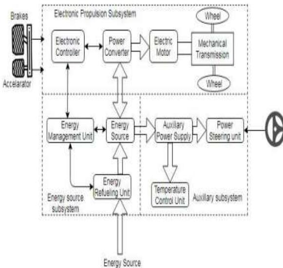
Fig. 1. Block diagram of an electric vehicle [13]
