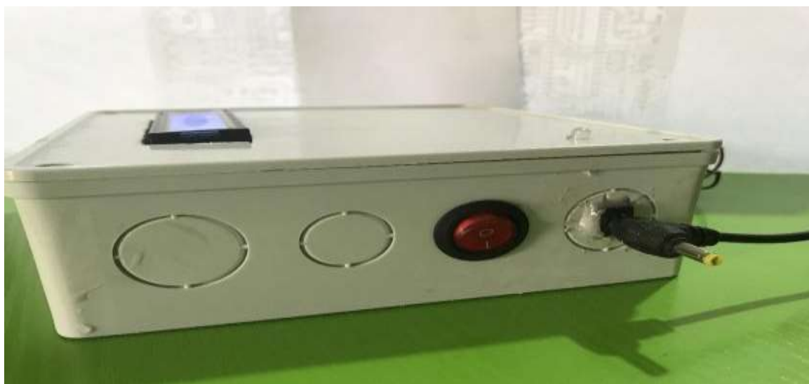
Figure 6: Side view of switch and adaptor power source
