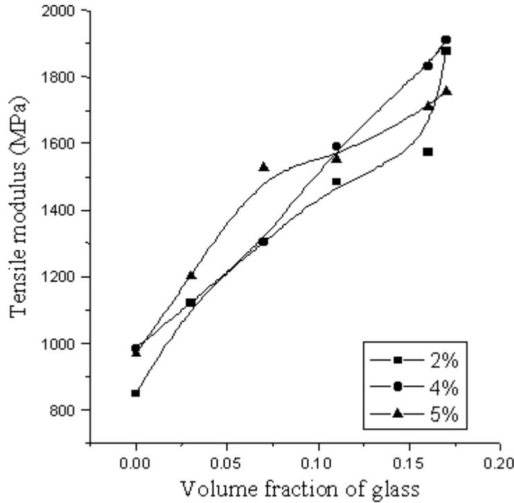
Fig. 2: Effect of glass volume fraction on the tensile modulus
