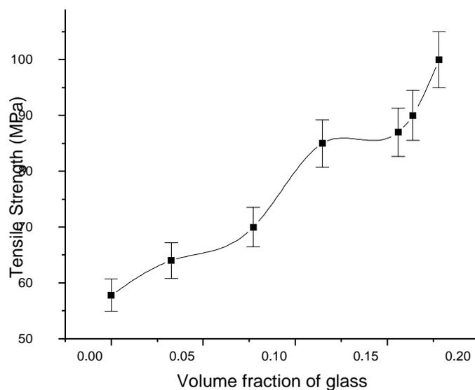
Fig. 3: Effect of glass volume fraction on the tensile strength
