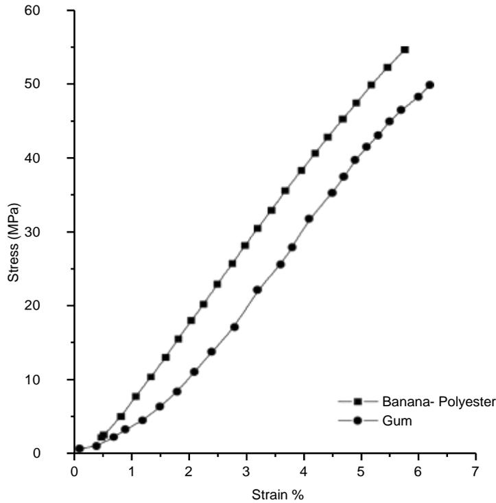
*Fig. 1: Comparison of the stress-strain behaviour of neat polyester and banana fibre composite*
