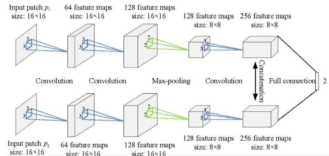
Figure 2: Schematic diagram based on CNN fusion algorithm
