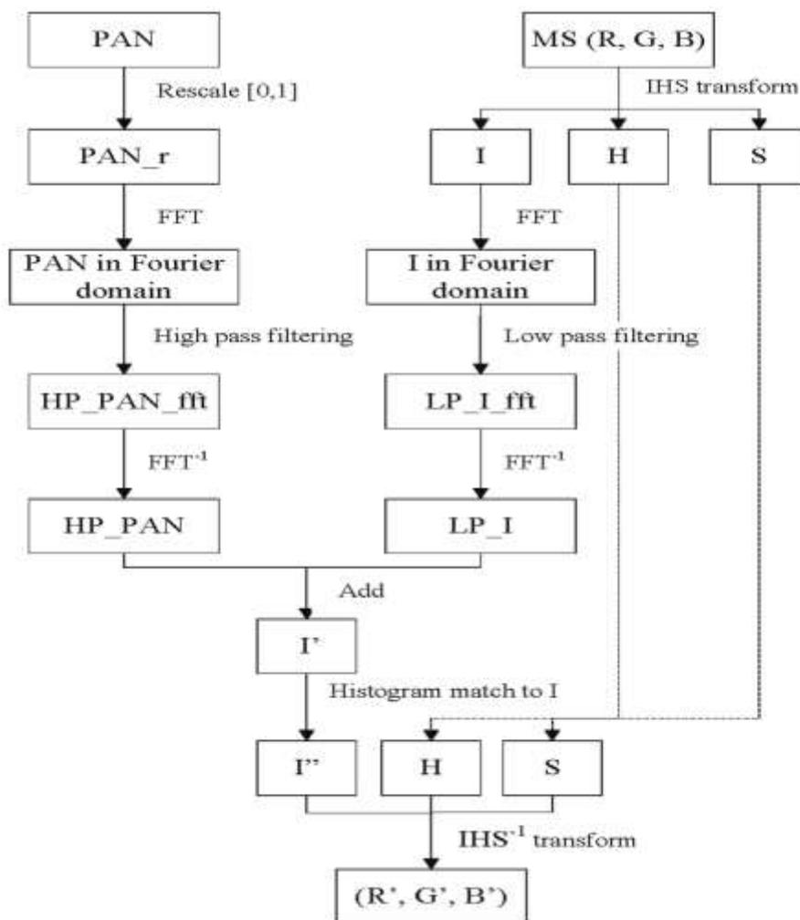
Figure 3: Framework diagram based on the IHS domain fusion method
