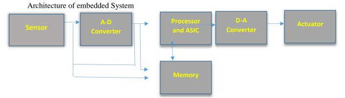
**Sensor**: Sensor converts physical quantity to an electrical signal & stores it in the memory.
