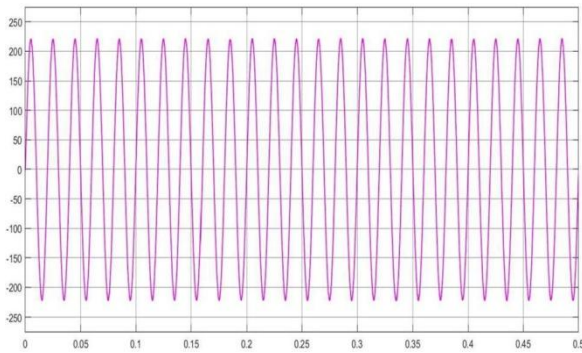
Fig. 5. Balanced grid current in phase-a
