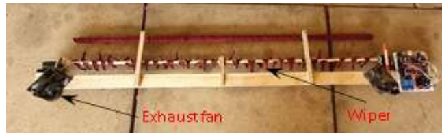
Fig4: Cleaning shaft of the proposed solar panel cleaner.
