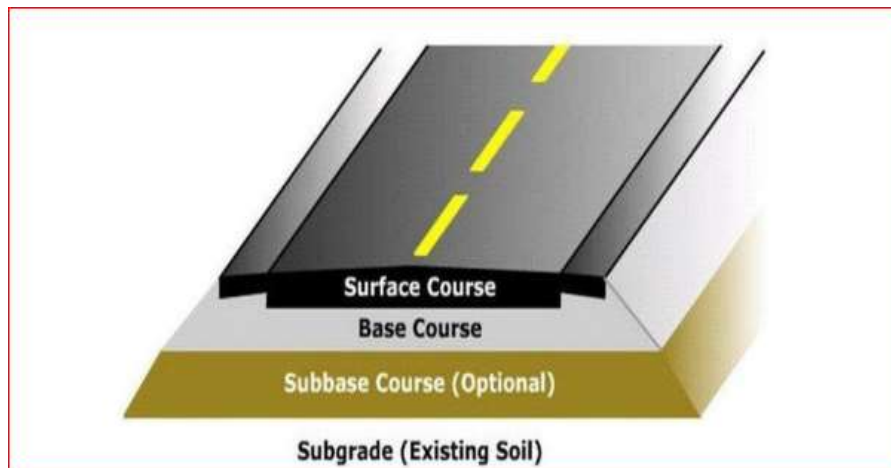
Fig 2: layers of flexible pavement
