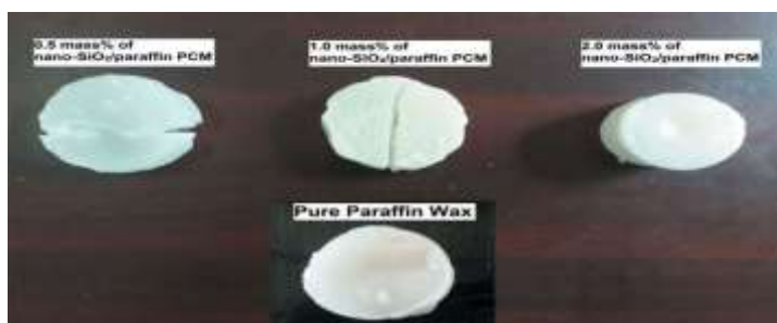
Figure 1. Photograph of the prepared nano-SiO 2 /paraffin PCM samples.
