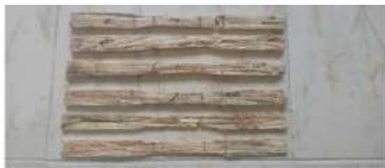
Fig.5. Specimen after tensile test
