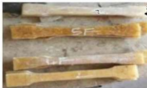
Figure 4 final epoxy resin bagasse composite
