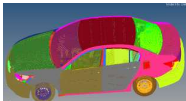
Figure 8 Displacement in Al-Mg material after side impact.
