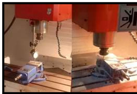
Fig.4 Experimental Setup of END Milling
