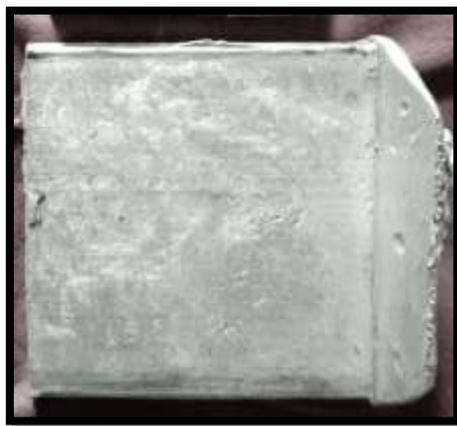
Fig. 1: Casted Aluminium SiC/Gr Composite
