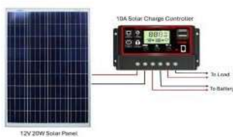
Fig 4 Solar Power Circuit
