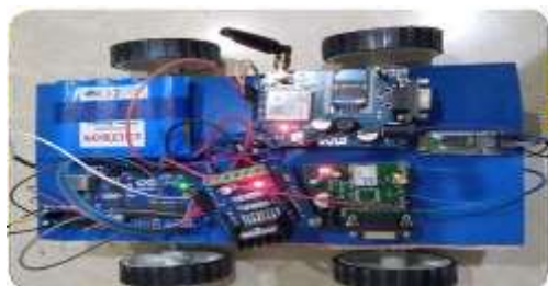
Fig. 4: AMS for Vehicle tracking and Accident Detection
