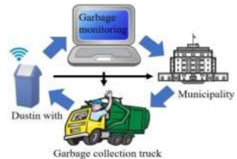
Fig. 1. Architecture for Garbage Monitoring and Collection System
