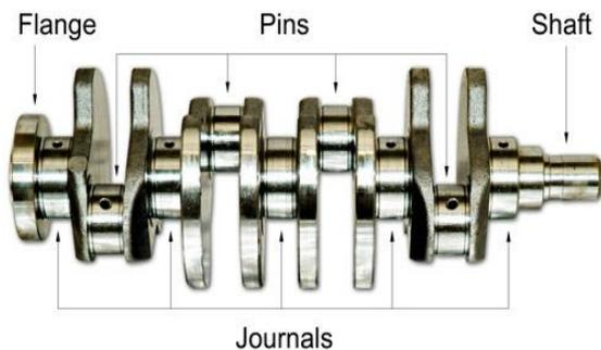
The crankshaft consists of the shaft parts which revolve in the main bearings, the crankpins to which the big ends of the connecting rod are connected, the crank arms or webs (also called cheeks) which connect the crankpins and the shaft parts.
