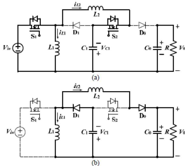
Fig. 3. Equivalent circuits of the proposed buck-boost converter in possible two states. (a) State 1. (b) State 2.
