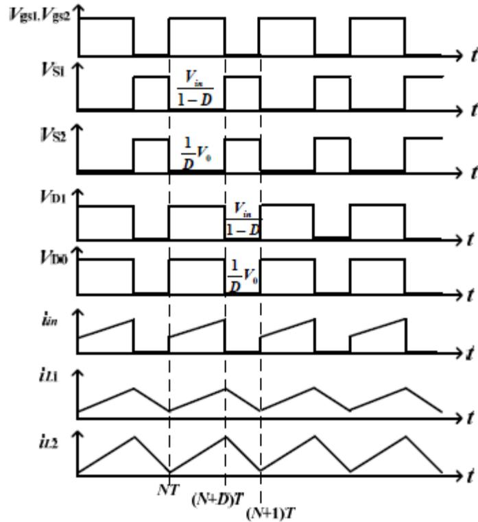
Fig. 2. Typical time-domain waveforms for the proposed buck-boost converter operating in CCM.
