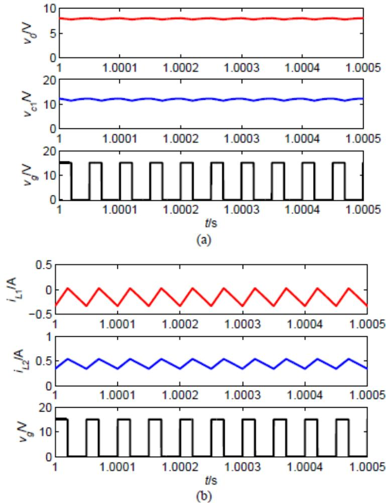
Fig. 6. PSIM simulations for the proposed buck-boost converter operating in step-down mode. (a)  $v_0$ ,  $v_{C1}$ , and  $v_g$ . (b)  $i_{L1}$ ,  $i_{L2}$ , and  $v_g$ .
