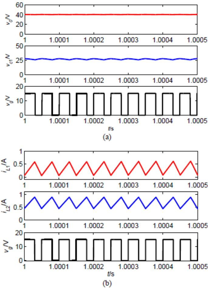
Fig. 5. PSIM simulations for the proposed buck-boost converter operating in step-up mode. (a)  $v_0$ ,  $v_{C1}$ , and  $v_g$ . (b)  $i_{L1}$ ,  $i_{L2}$ , and  $v_g$ .
