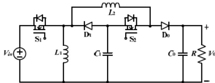
Fig. 1. Proposed transformerless buck-boost converter
