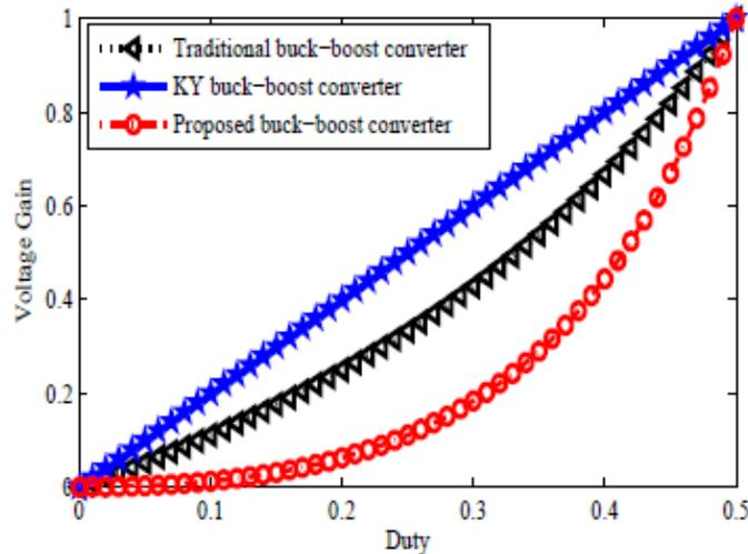
Fig. 4. Comparisons about the voltage gain among the traditional buck-boost converter, the KY buck-boost converter, and the proposed buck-boost converter. (b) Step-down mode.
