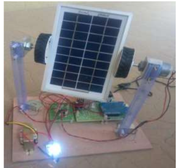
sensing device will be processed by the microcontroller and the microcontroller drives the DC Servo motor in the desired direction.
