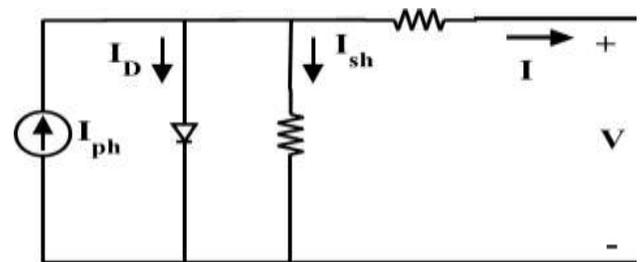
Fig.6. Equivalent Circuit of Single Diode Modal of a Solar Cell
