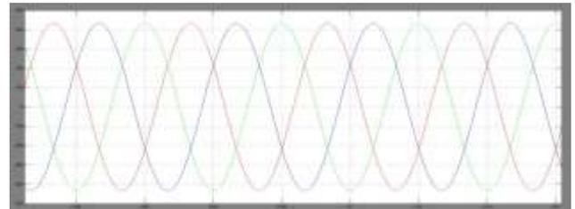
Fig.10. Simulation Wave Form of Response of AC Bus Voltage with STATCOM
