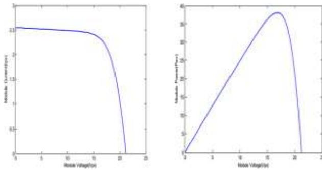
Fig.7. V-I & P-V Characteristics of a 36w PV Module
