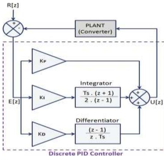
Fig.5. PID Controller Schematic
