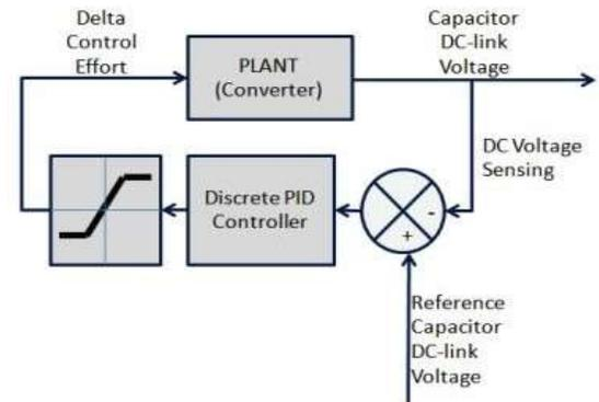
Fig.3. DC Capacitor Voltage Control
