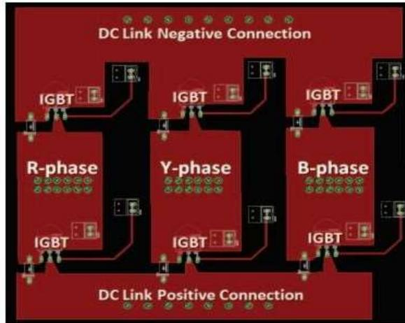
Fig.1. PCB Layout of Power Circuit
