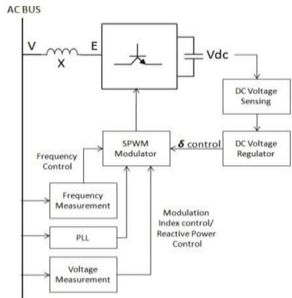
Fig.2. STATCOM with its Control Systems
