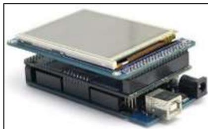
Figure 7: Arduino MEGA with SainSmart C46 LCD kit
