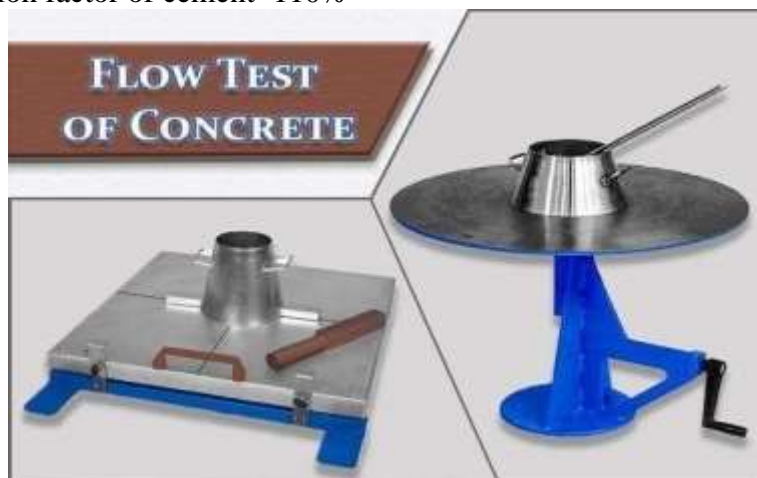
Fig 9: Flow Test on concrete
