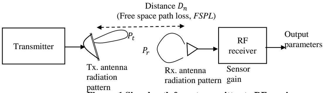
**Figure. 1 Signal path from transmitter to RF receiver**
