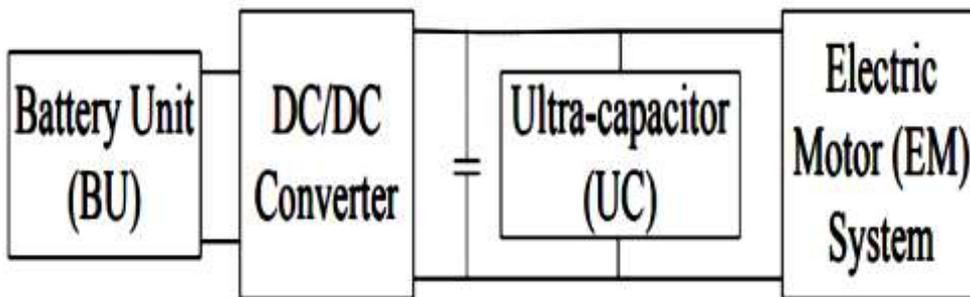
**Fig:1 Proposed partially de-coupled H-Energy Storage System with directly coupled UC with DC bus**
