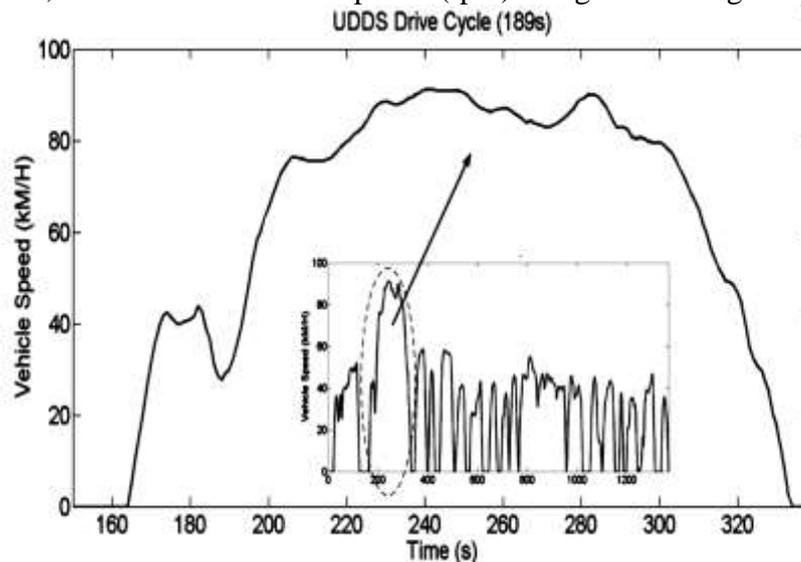
**Fig:5 UDDS drive cycle and zoomed-in view of the 189 seconds of UDDS drive cycle used in the study**
