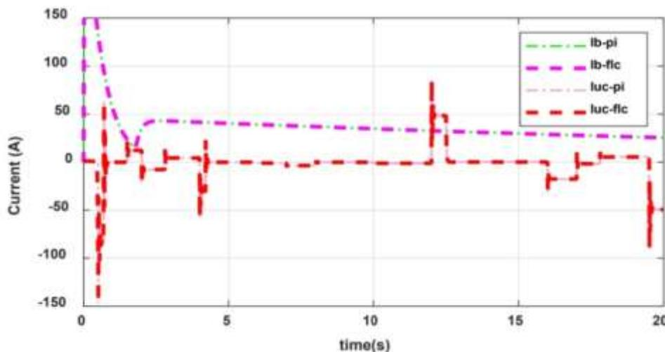
**Fig:9 Battery unit Discharging Current(PINK), Ultra capacitor discharging Current(RED)**
