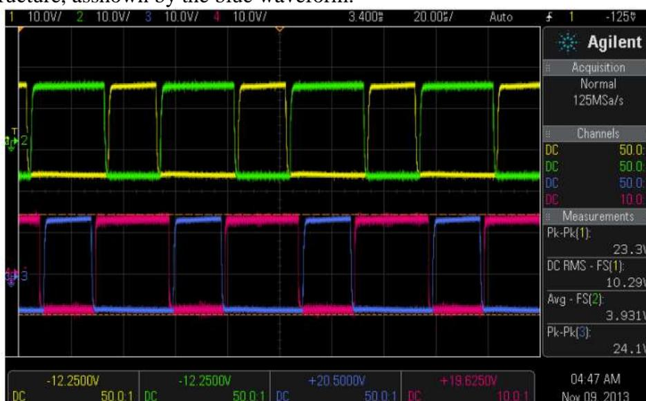
**Fig:7 Boost switch PWM signal in module-1 (Yellow), Buck switch PWM Signal in module-1 (Green), Boost switch PWM signal in module-2 (Blue), Buck switch PWM signal in module-2 (Pink).**
