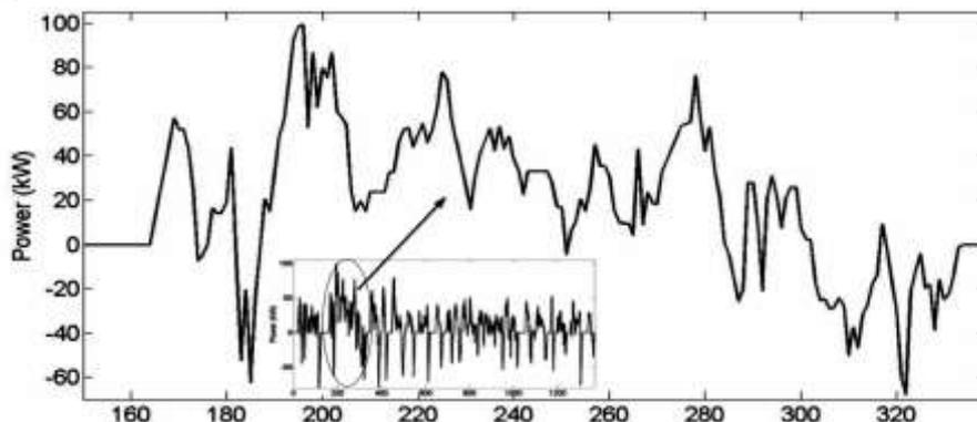
**Fig6: Powerprofile of Teslamodel S on the UDDS drivecycle and the zoomed-inview of the power during the 189seconds**
