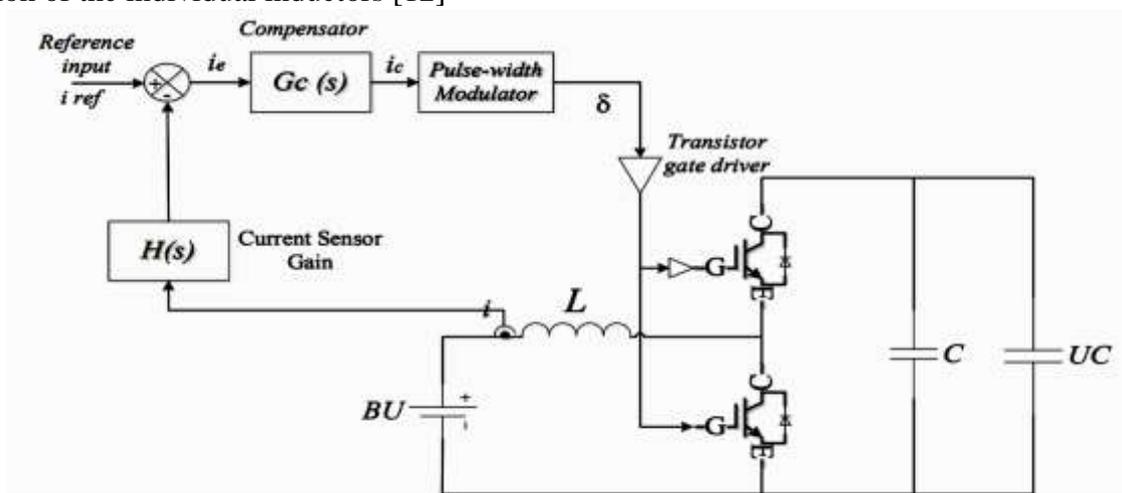
**Fig 4: Schematic diagram of Individual Inductor's Current Regulation**
