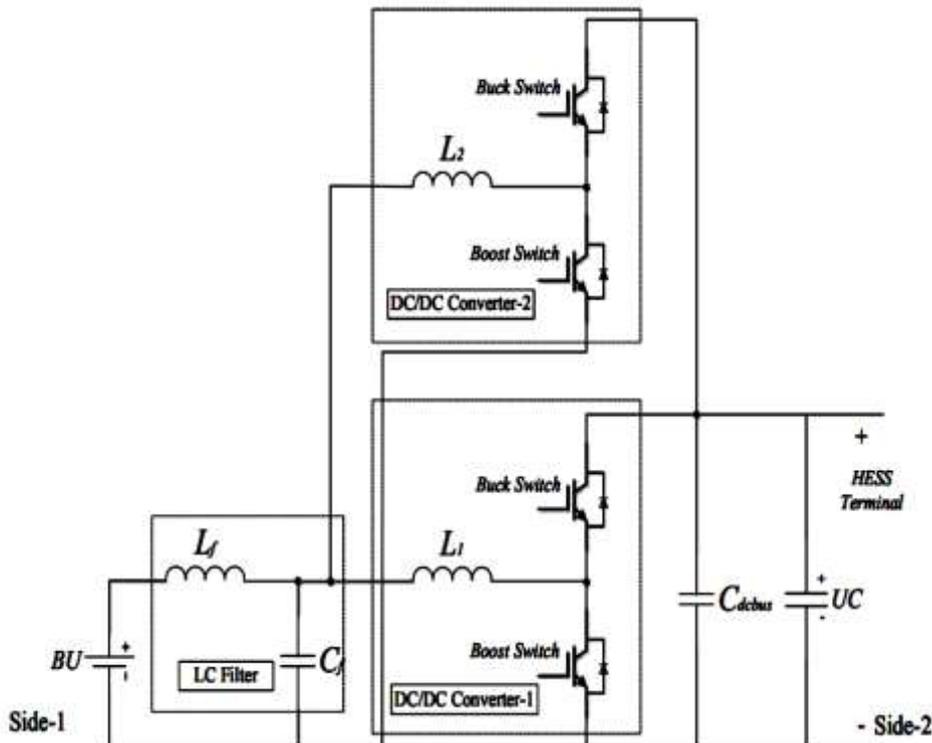
**Fig:2 two module interleaved bi-directional buck boost dc to dc converter**
