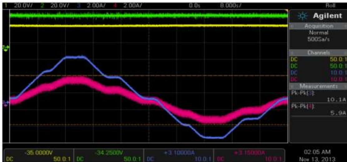
**Fig:8 Results of Battery discharging current from proposed model (blue), inductor current from proposed model(pink), battery terminal voltage from proposed model (yellow), ultra-capacitor terminal voltage (green)**
