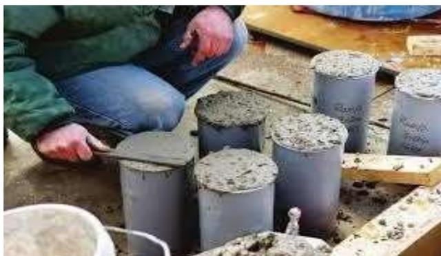
**Figure-10: Concrete specimen**
