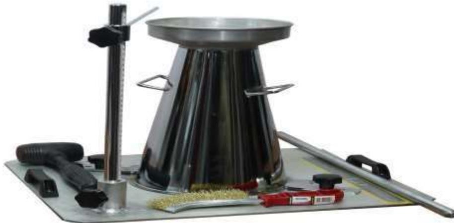
Figure-7: Concrete Slump Test
