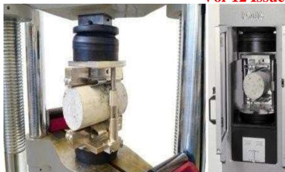
**Figure-10 Split Cylinder Testing Machine**
