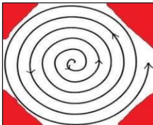
Spiral algorithms have trouble reaching the corners and are unable to clean the room's corners, whereas the random walk algorithm can reach any corner. Random walk can clean whole room whereas spiral algorithm can clean only 80% of the room. As a result, the random walk method outperforms the spiral algorithm.
