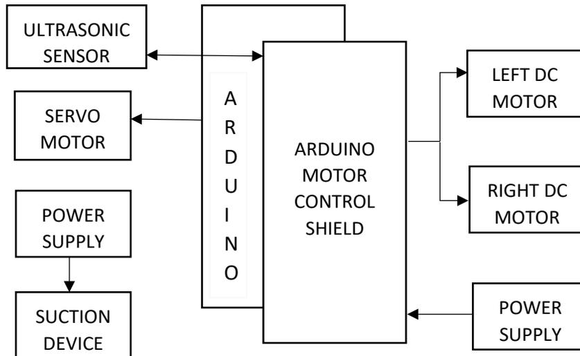
The proposed robot is a battery-operated electronic device with an ultrasonic sensor which is directed by a servo motor generates binary data. This data is then transferred to the control unit, i.e., Arduino, which is considered the robot's brain. Based on information provided by the sensor, this unit generates control signals automatically. Finally, the wheel motor drivers get these control signals.
