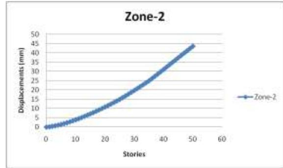
Fig-11: Maximum displacement that occurs at top storey is 43.484 mm
