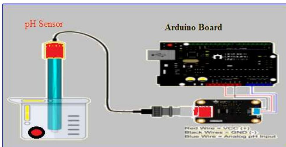
Fig.no.1 pH sensor Interfaced with Arduino Uno Board
