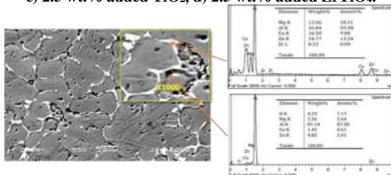
Fig. 7 SEM-EDS analysis of 2.5 wt.% ZrO<sub>2</sub> added 7075 aluminum alloy.
