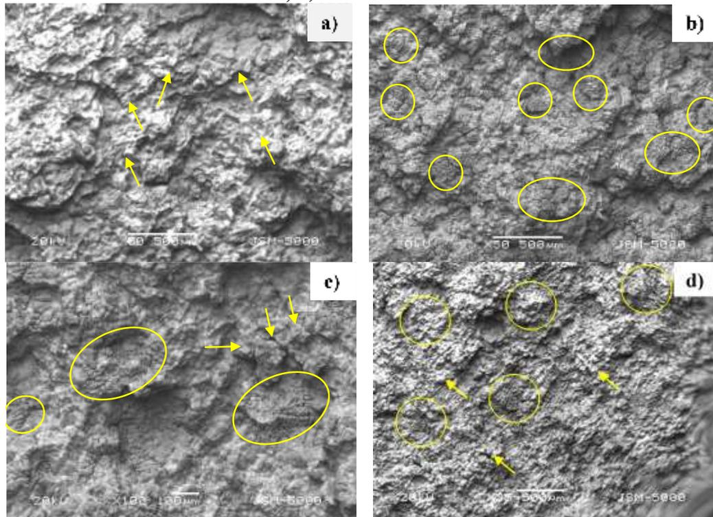
Fig. 6 Fractography analysis (SEM-BSE mode) of Al 7075; a) as-cast, b) 2.5 wt.% added ZrO<sub>2</sub>, c) 2.5 wt.% added TiO<sub>2</sub>, d) 2.5 wt.% added ZrTiO<sub>4</sub>.
