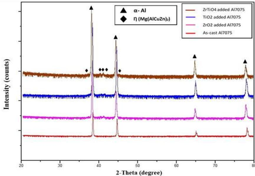
Fig. 8 XRD analysis of Al 7075; a) as-cast, b) 2.5 wt.% added  $\text{ZrO}_2$ , c) 2.5 wt.% added  $\text{TiO}_2$ , d) 2.5 wt.% added  $\text{ZrTiO}_4$ .
