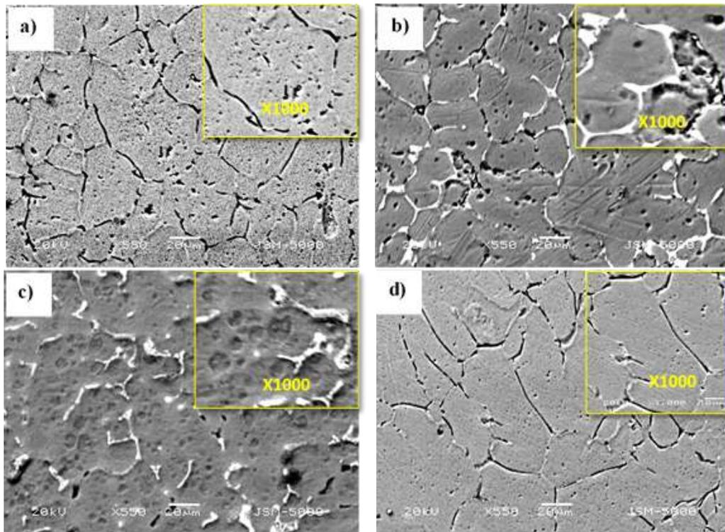
Fig. 4 the SEM micrographs of 7075 aluminum alloy; a) as-cast, b) 2.5 wt.% added  $ZrO_2$ , c) 2.5 wt.% added  $TiO_2$ , d) 2.5 wt.% added  $ZrTiO_4$ .
