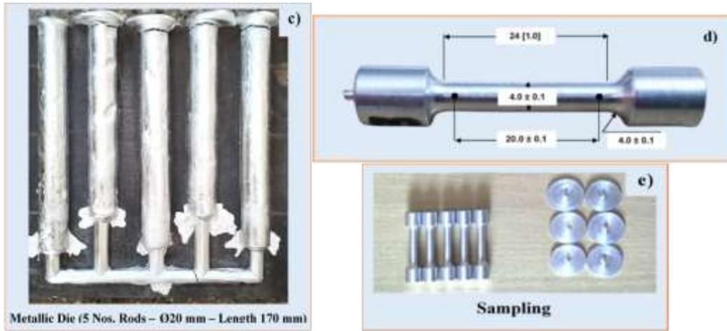
Fig. 1 Experimental set-up and sampling plan a) resistance heating furnace; b) metallic die dimensions; c) cast sample dimension; d) tensile specimen dimensions as per ASTM E8M; e) sampling.
