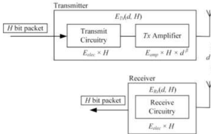
Figure3: Energy Consumption Model
