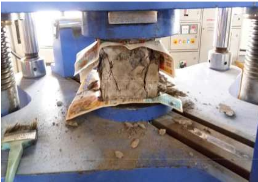
Figure 3.2 Testing compressive strength of cube
