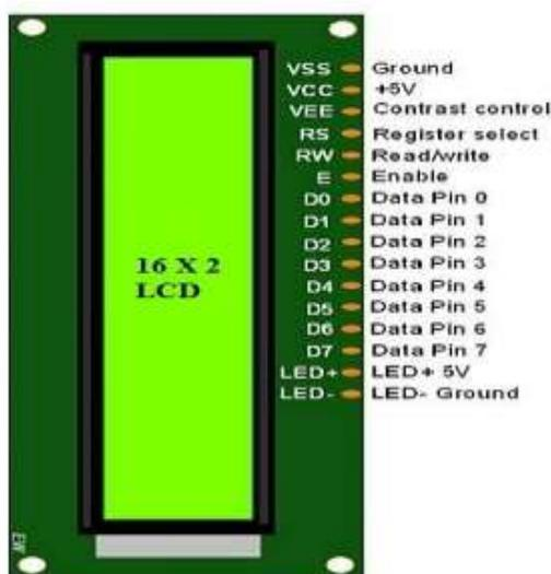
Fig 7: LCD-16x2-pin-diagram
