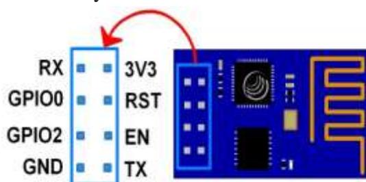
**Fig 6:**ESP8266 Wi-Fi Module Pinout
