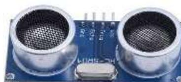
Fig 4: Ultrasonic sensor
