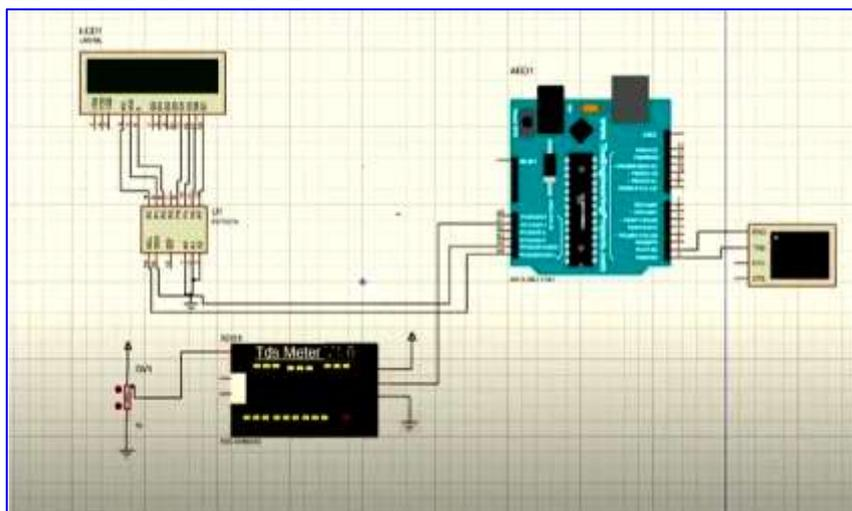
**Fig.no.2 Simulation using Proteus Software for TDS Sensor**
