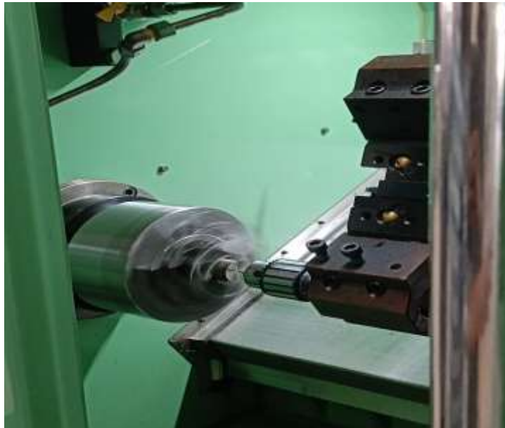
Fig 1 Central Drill Operation in CNC Lathe
