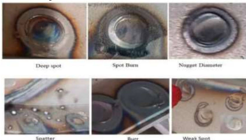
Figure 3: Defects in resistance spot welds
