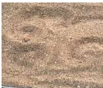
Sample of fine aggregates
