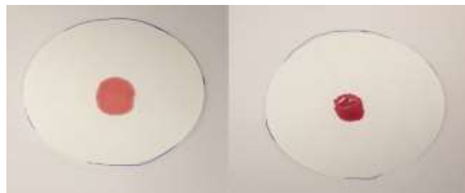
Figure 3: Representative images from 2 cases, with the dropper method in a controlled environment, with the image on the left having a PCV of 0.05 L/L [5%], and on the right a PCV of 0.45 L/L [45%]
