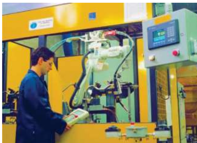
Fig. 9. Lead-through programming by teach pendant.
