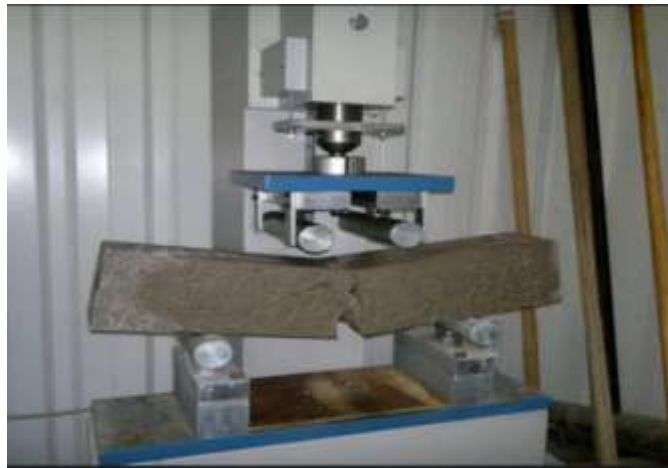
Fig:12 Flexural strength test apparatus
