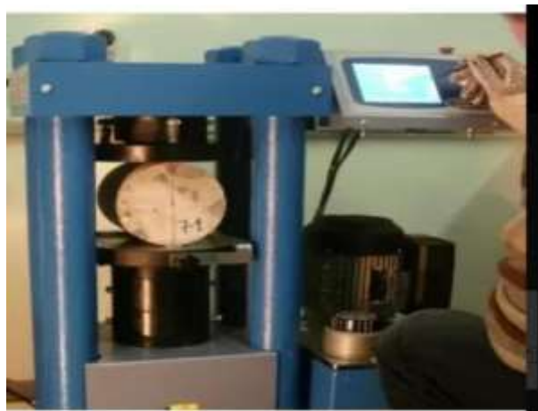
Fig: 11 Split tensile strength test apparatus
