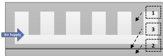
Fig. 1. A cross-sectional illustration through a typical bending SPA featuring a ribbed morphology.
